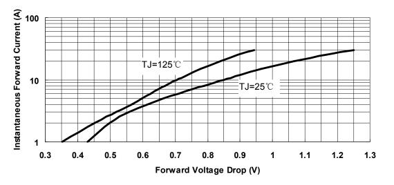
Fig.3-Typical Instantaneous Forward Voltage Characteristics
